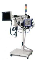
A basic base can be customized to accommodate Nordson equipment, including pumps, melters, guns and wire harnesses. Customer options include: adjustable feet or casters; fixed or pivotable control mounting; and short or long arms.
