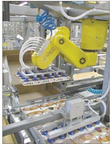
Automate your end-of-line process with this robotic packer palletizer for the ultimate in flexibility for your packing needs.
