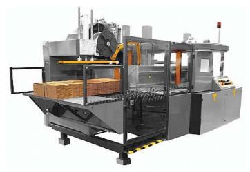
ISB Mono is available in four model sizes and can handle stacks from  $170 \mbox{ mm}$  to  $1800 \mbox{ mm}$  wide.
