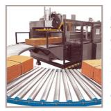
By squaring the stacks, a higher standard of pack quality is achieved which is ideal for load forming, especially where fully automatic palletising equipment is in use. Irregular bundles which interrupt the palletising process due to positioning problems are eliminated.
