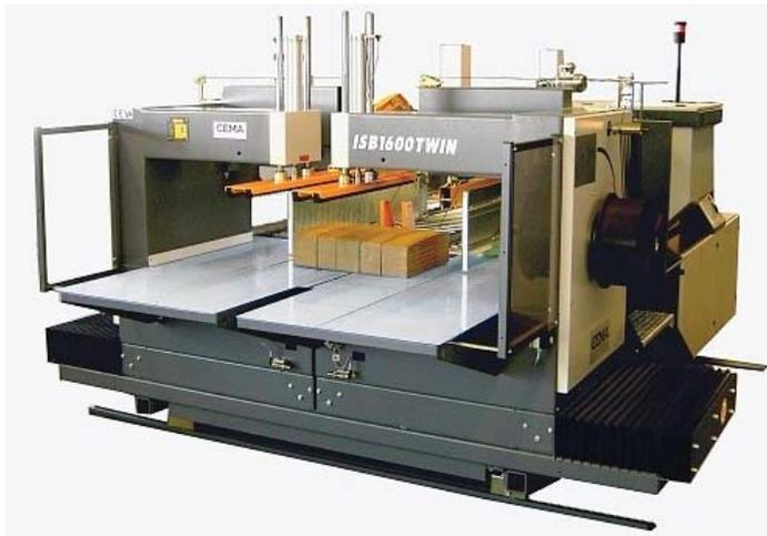
The ISB Twin operates with a two head strapping system and offers the ultimate in operational flexibility, efficiency.
