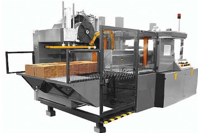
ISB Mono is available in four model sizes and can handle stacks from 170 mm to 1800 mm wide.
