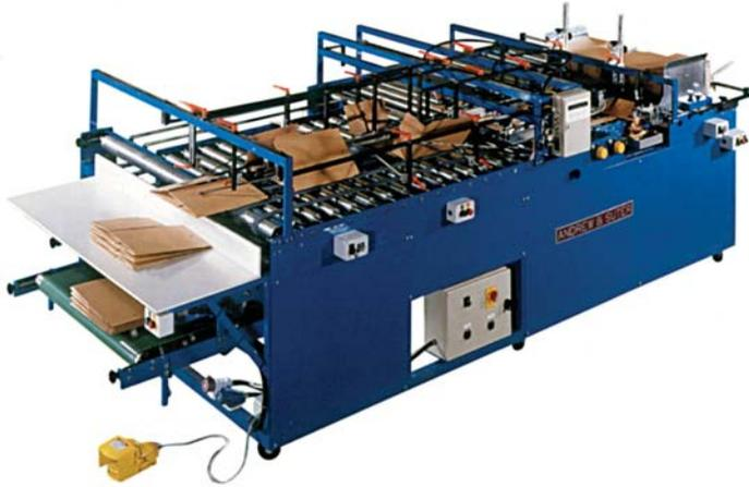
This MultiNova Gluer is a multi-purpose gluing machine which can handle carton board, F, E, B and C flute corrugated including doublewall straight line gluing. The machine can glue:
