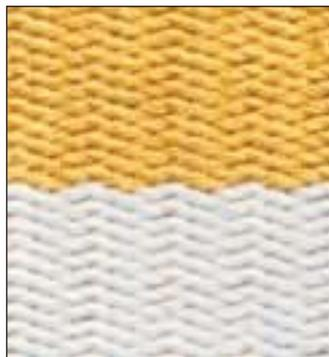
layer of aramid fibres is firmly woven in to reinforce the surface of the belt.
