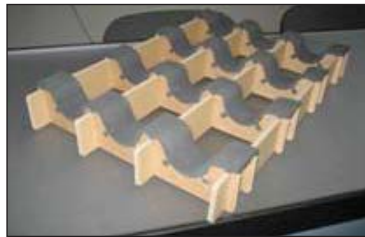
x. tara clip: The contour specific forms are clip in pads with heat resistant connections and are exchangeable by wearing out in lays.
