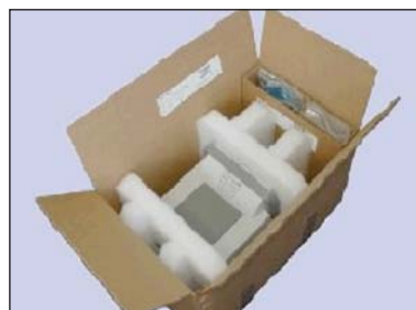
iv. tara set: They are either complete or confectionery package, customized sizes made from HKP, corrugated board, foam, VCI-foil, labels, etc.
