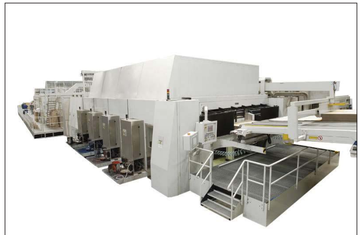
Rapidex (Bobst Group), is dedicated to the design of large size flexo converting machines with in line slotting and rotary die-cutting.
